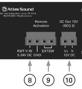
10. DC Output – The ECS-3 can handle 15A of current before the breaker opens. If 15A is not enough current to support the power requirements, this output can be used to activate an additional power outlet such as the ECM-20SH. This triggered 12VDC voltage works in conjunction with Sequence 3 timing section. Contact Atlas Sound for AC outlet options. Note: This DC output can also be used to power an LED indicator for a remote activation switch such as the Atlas ECS-KSW3.
